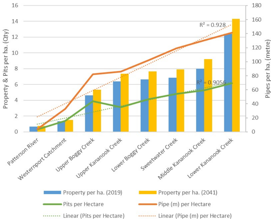
Figure 5: Infrastructure Required per Hectare
