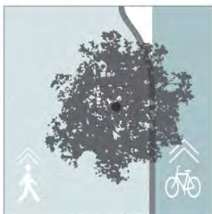
Walking & bike paths physically separated by kerb, and visually contrasting surface materials.
