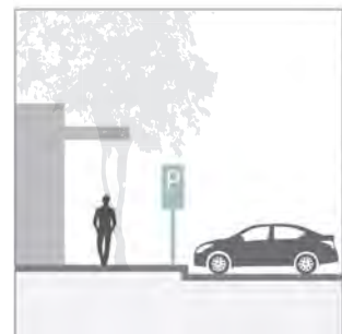
Car Parking Signage is clear of obstructions.
