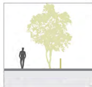
Bollard protection in kerbless environment
