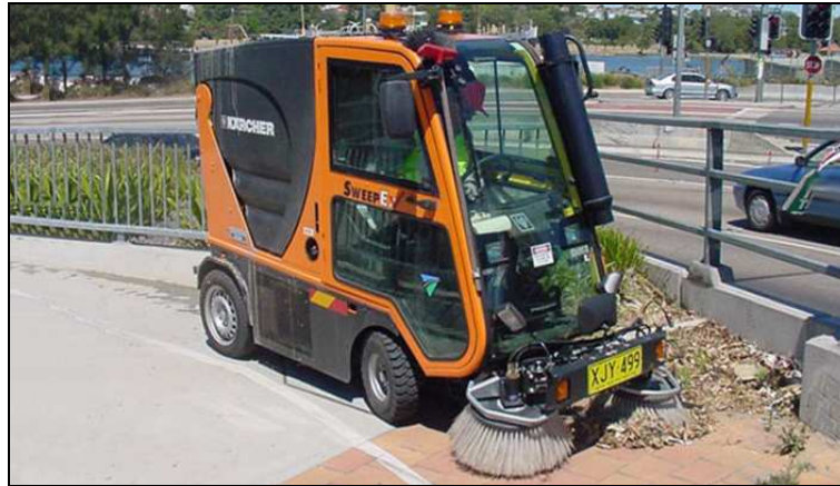
Figure 7.12 Bicycle path sweeping machine as used in NSW Source: NSW Bicycle Guidelines
