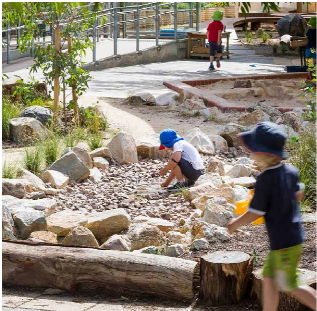
Water play run-off can be directed to dry-creek swale areas & used to passively irrigate planting, also providing interactive spaces for play
