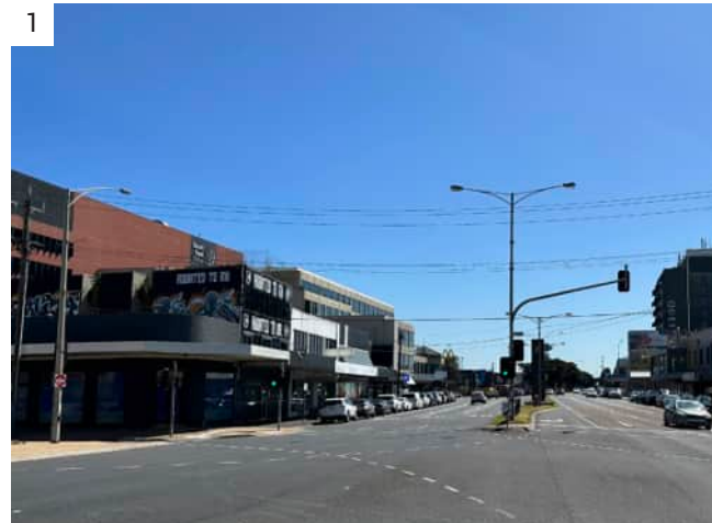
1 Nepean Hwy CBD intersections Existing lighting consists of tall Vicroads light poles located on the centre median, with additional light poles at intersections. These lights provide functional illumination to the roadways and footpaths.
