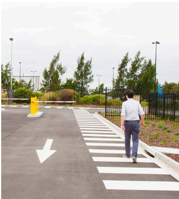
Clearly defined pedestrian pathways are important within car parks to avoid potential pedestrian vehicle conflict
