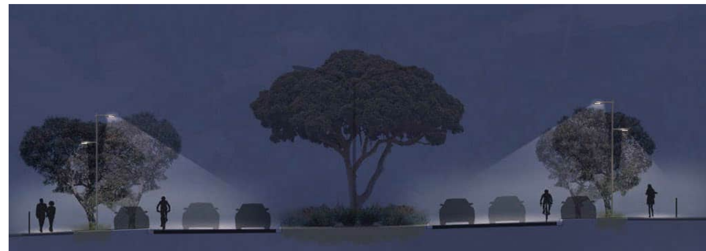
Proposed lighting scheme with new vehicular and complimentary pedestrian lighting to improve functionality and safety.
