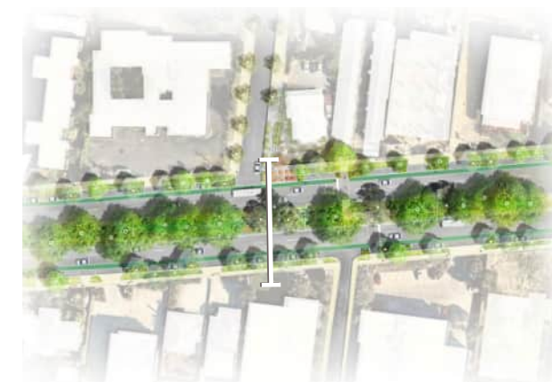
Existing cross sections illustrates the wide central median with a western crossfall to Kananook Creek as well as a consistent two lane carriageway throughout the precinct. Existing cafe at Fiocchi Avenue
