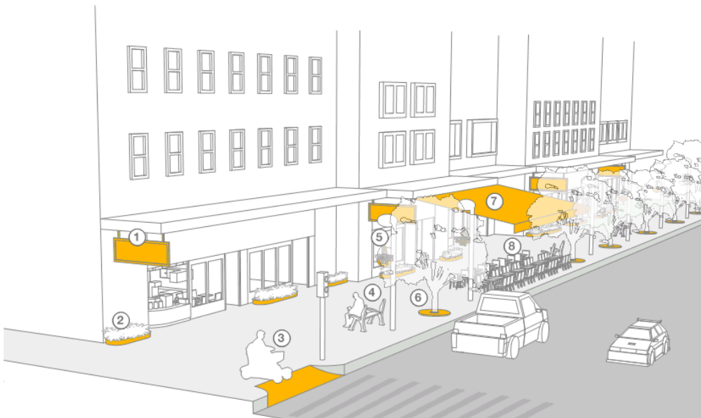
Street Design Features for Active Frontage
