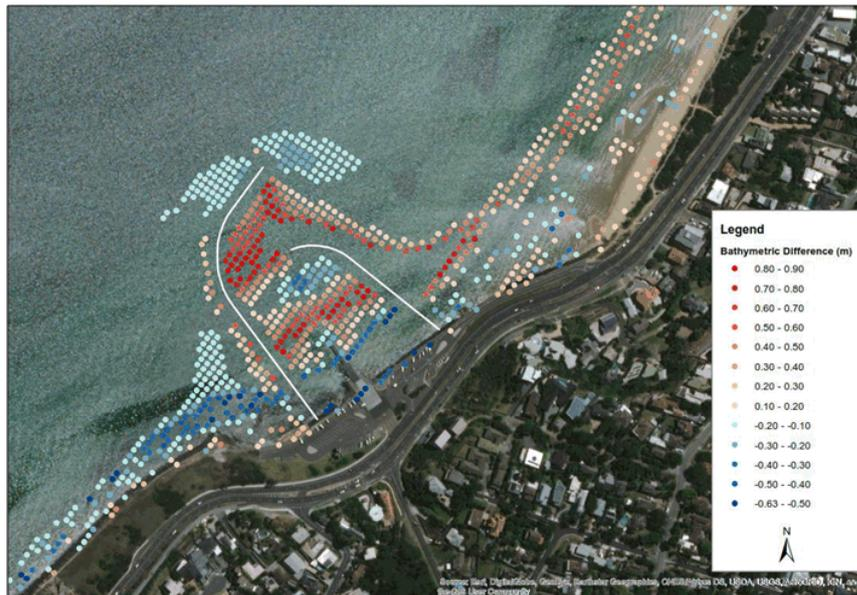
Figure 6.4 Difference in Bathymetry for Developed – Existing Scenario, Annual Winds
