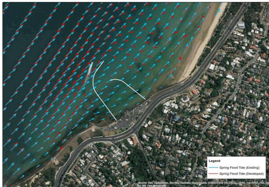
Figure 6.2 Spring Flood Tide Current Vectors for Developed and Existing Scenarios.
