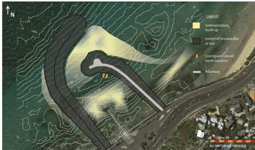
**Figure 6.5 Areas of Sediment Deposition as Predicted by the Modelling**
